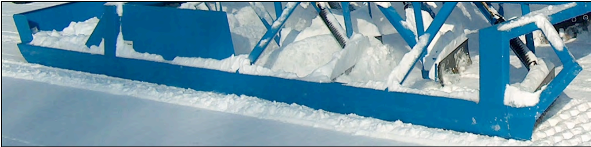
Photo 2.4 Side rail on a multi-blade drag helps keep snow contained within the drag.
