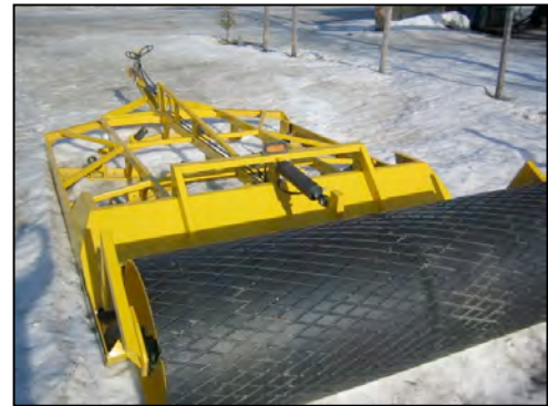
Photo 2.16 Typical rear drum roller assembly
