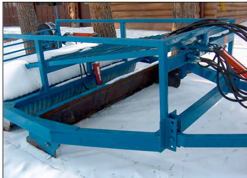
Photo 2.19 Typical single cutting blade
