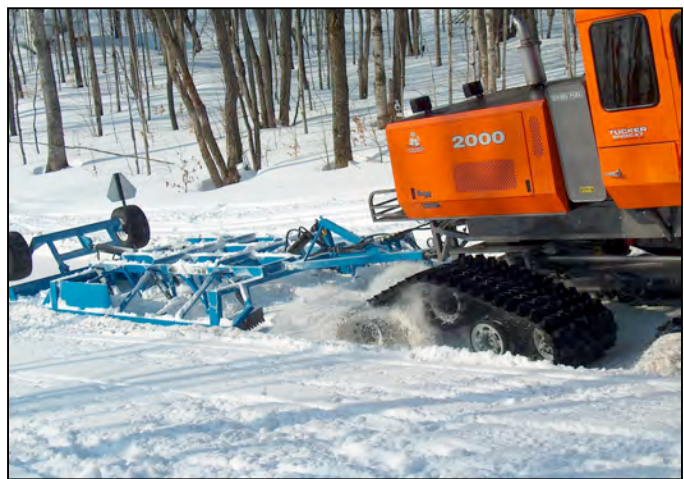
Photo 4.13 Beware of trenches dug by spinning tracks
