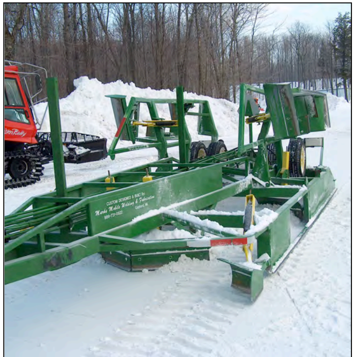
Photo 2.2 Drag with hydraulic wings
