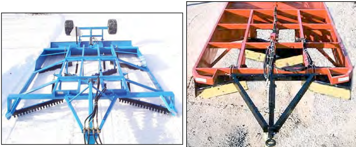
Photo 2.3 Typical multi-blade frames and blade configurations
