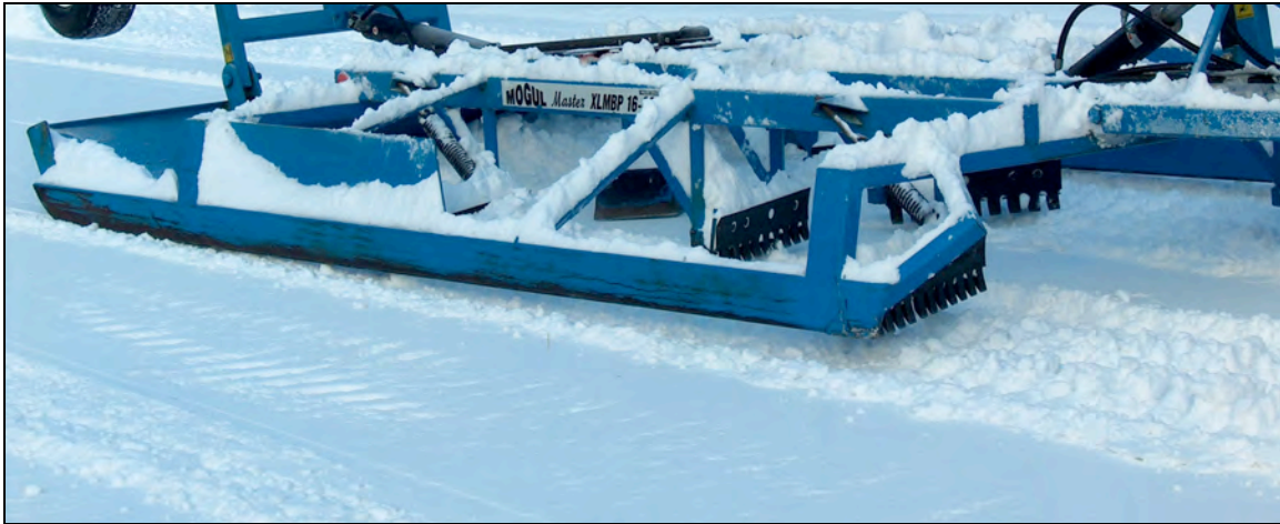
Photo 4.10 Use only the rear set of blades to groom minimally moguled trails.
