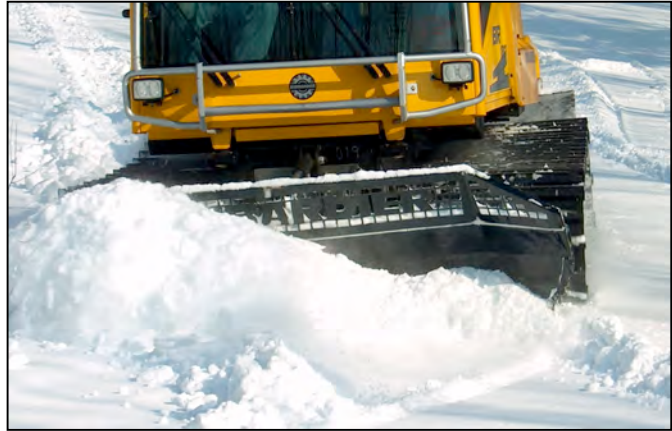
Photo 2.29 Typical front blade at work
