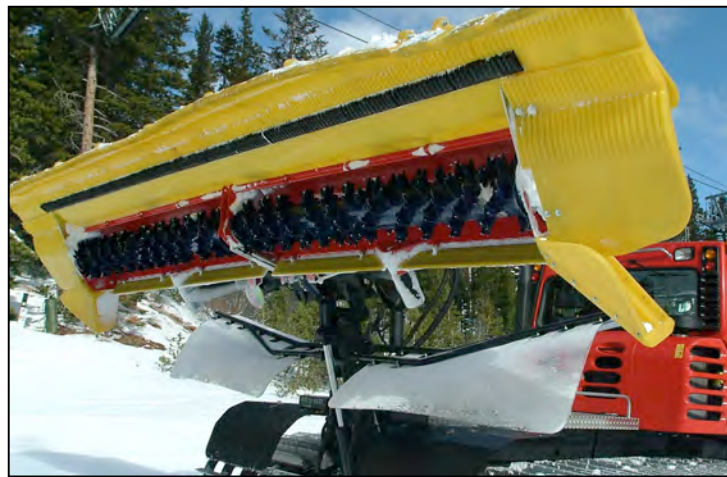
Photo 2.21 View of the underside of a tiller
