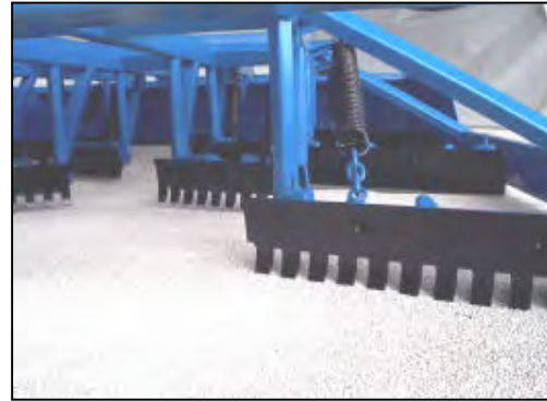
Photo 2.8 Serrated cutting blades
