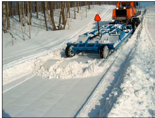
Photo 4.3 Remove back up piles! Use SMV sign.
