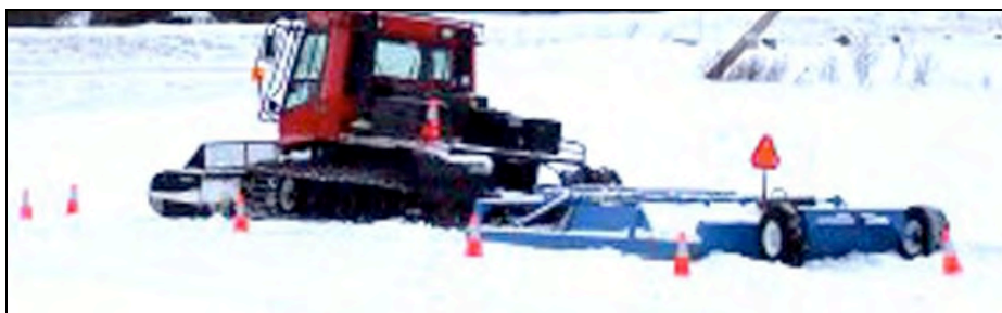
Photo 3.3 Place cones or other warning devices around and in advance of a groomer that has broken down on the trail and must remain there for an extended period.
