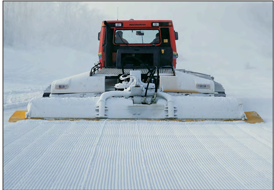
Photo 2.20 Typical rear-mounted tiller
