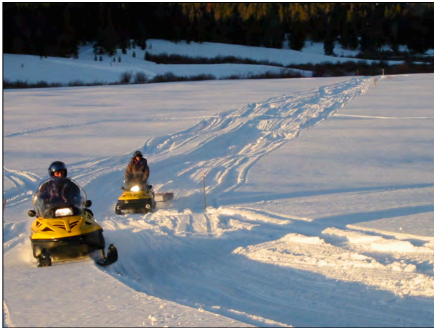
Photo 1.1 Snowmobile traffic creates rough trails that require trail grooming
