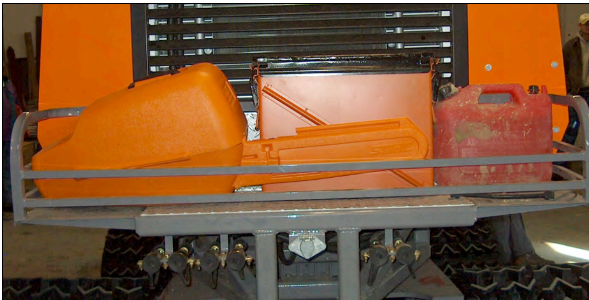
Photo 2.30 Typical cargo deck used to carry tools, spare signs, and spare fuel
