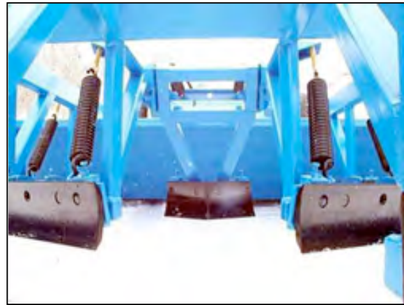
Photo 2.5 Spring tripping blades
