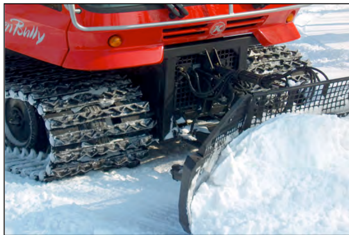
Photo 4.15 Watch behind the front blade to monitor blade height relative to track location
