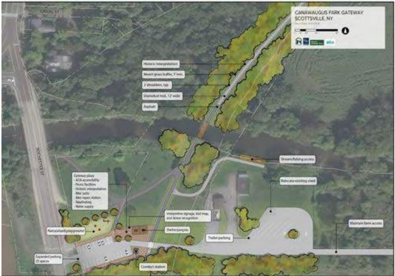
Conceptual Canawaugus Park Gateway in Scottsville provides parking for vehicles and trailers, and also offers improved trail access and amenities to trail users
