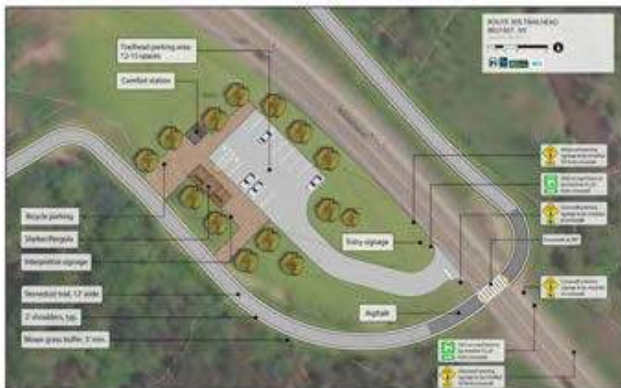
Proposed typical Trailhead illustration for the GVG crossing at Route 305. Shows typical parking and trail amenities such as a shade structure, benches, bike racks, comfort station and wayfinding. Safety and crossing improvements are provided for an improved road crossing.
