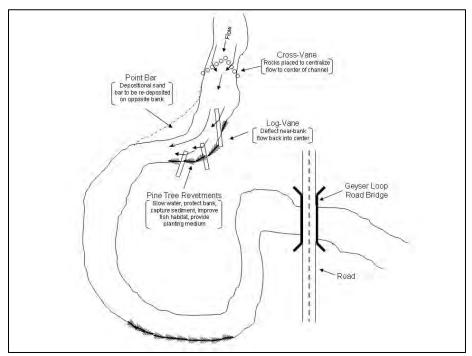
Figure 21 Geyser Brook Erosion Control
