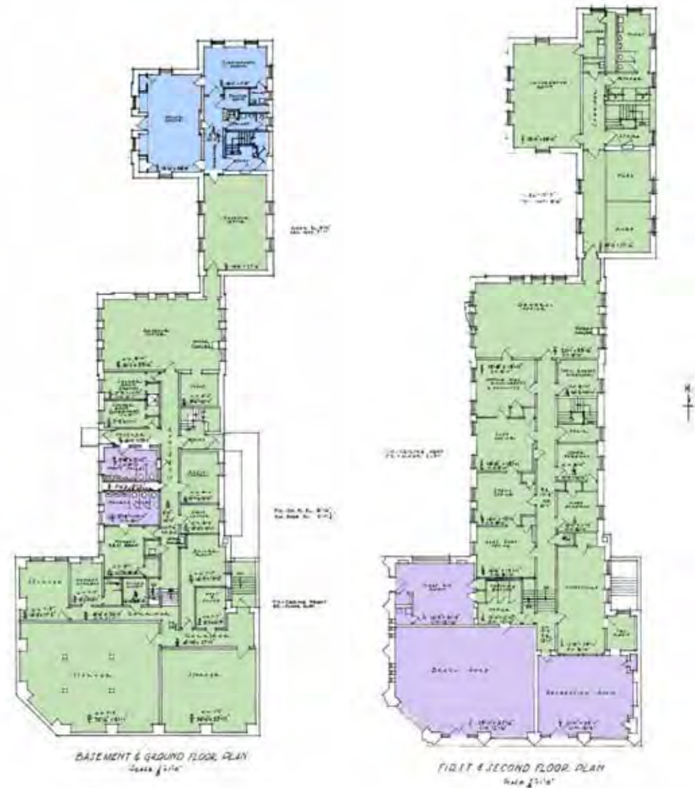
Administration Building Floor Plans c. 1950 Highlighted areas (green) is office spaces, (blue) is police offices and (purple) is public areas.
