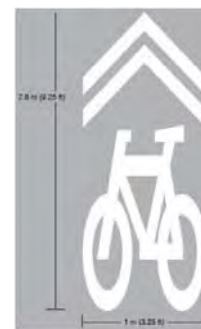
Shared lane marking
