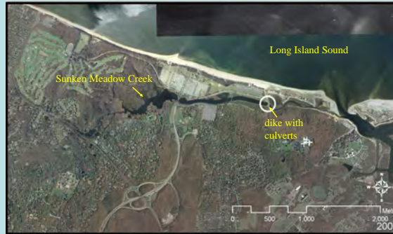
Changes in Sunken Meadow Creek and the landscape over time (1930 vs. 2007) The creek channel was moved, dredged, and a dike was constructed during park expansion in the 1950's.
