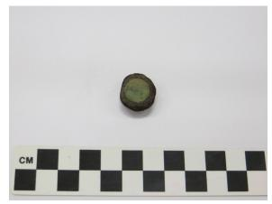
**Crushed lead pipe**
