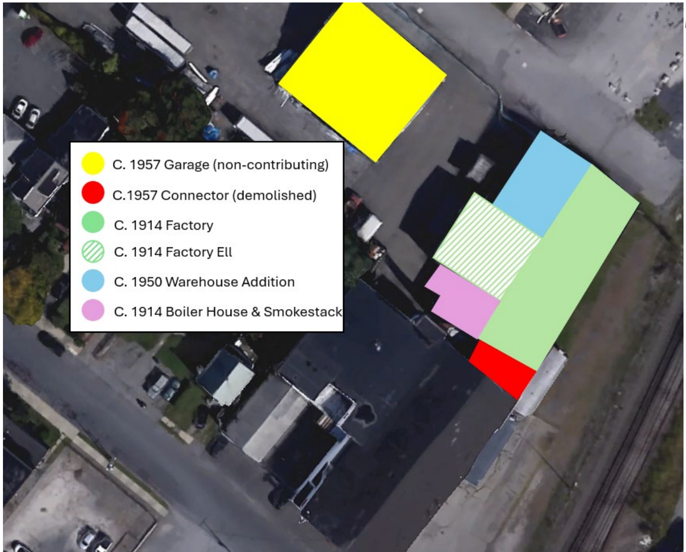
Figure D: Kingston Barrel Factory building chronology plan. Note: The connector was demolished in 2023 and the Kingston Barrel Factory is no longer connected to the Warehouse. (Source: Google Maps)
